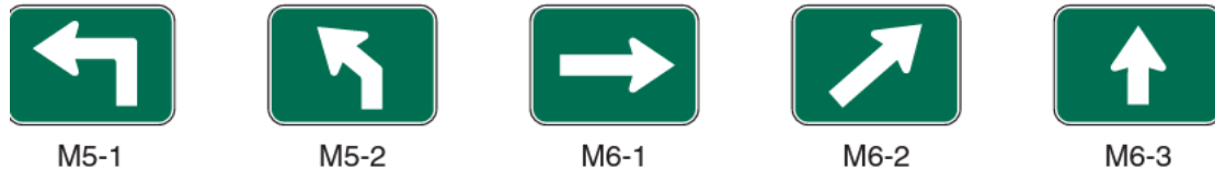
Advance Turn and Directional Arrow Auxiliary Signs for use with General Information Signs
